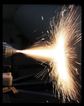
Metallization of all types of Babbitt alloys, and hard alloys, and repairing by metal-spray and hard chrome plating. This section has spraying and devices for thickness measurement and surface roughening. Also, Grinding and lathing operations will be metal-sprayed afterward
